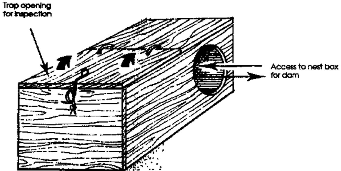
**Note:** In hot climates the top of the box can be made of wire mesh.
