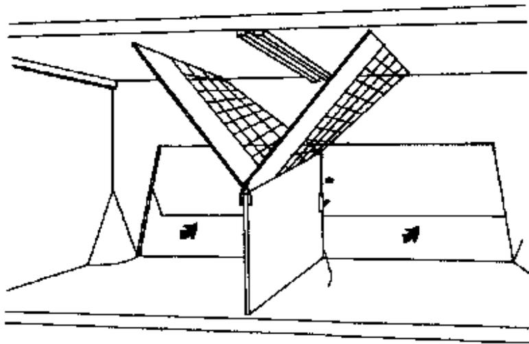
*FIGURE 27 Swinging rear wall in concrete hutch for waste removal (b)*
