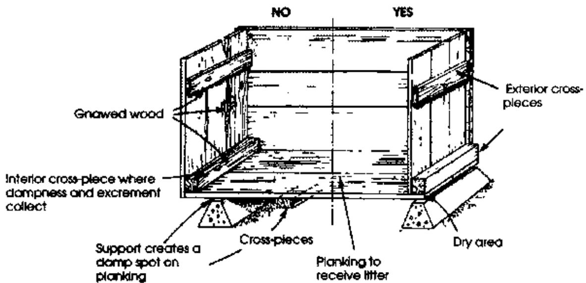
**FIGURE 26** Examples of correct and incorrect cage assembly, fostering good hygiene and resistance (b)
