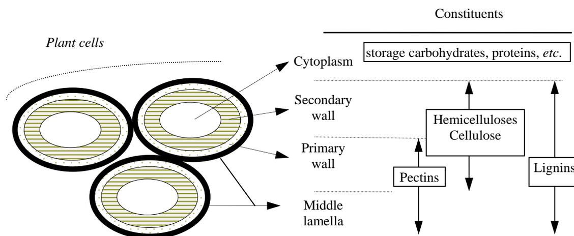
**Figure 1:** Schematic representation of plant cell walls, and their main constituents
