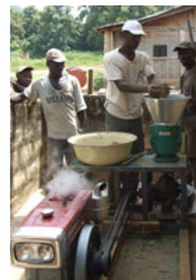
Figure 4 : *First use of the pelleting machine*
