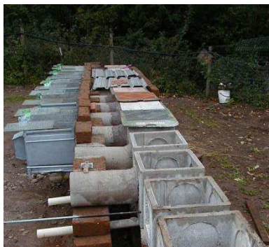
Figure 1: Building an underground cell system. A tube is connecting cells (right) with cages (left).
